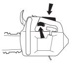
Note! Pull the front hand guard towards the front handle. The chain brake is now disengaged. Your saw is ready for use.
